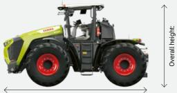
Overall length without front and rear linkage: 7760 mm
