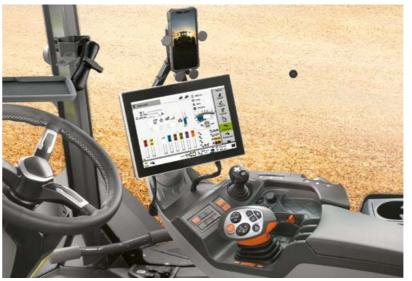
▲ CEMOS enables even inexperienced drivers to operate both tractor and implement as efficiently as possible throughout their entire shift. The operator assistance system offers continuous guidance – from ballasting and tyre pressure before you start work, to optimising the engine and transmission settings while work is underway.
