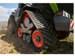
◆Two belt widths (914 mm or 762 mm) guarantee maximum ground protection. With the narrower track belts, the overall width of the XERION is less than 3 m.
