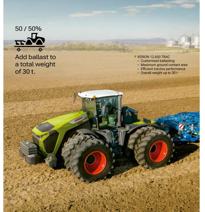
Less ballast, less ground pressure, lower costs. CEMOS helps operators select the right ballast before they leave the yard.
