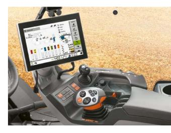
User-friendly operation, intuitive machine settings and unmatched ease of use with the CEBIS on-board information system and CMOTION multifunction control lever.
