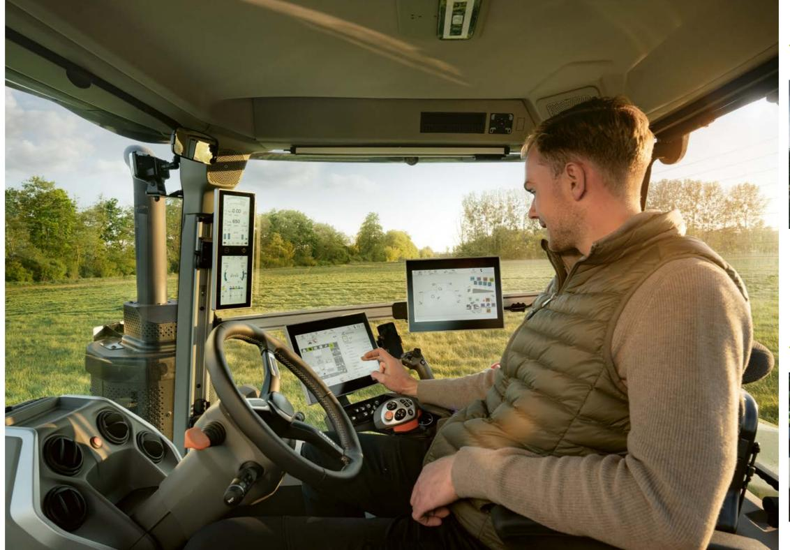
▼ The new AgXeed VCU (Vehicle Control Unit) automatically performs preplanned tasks so that the operator can concentrate fully on monitoring.
