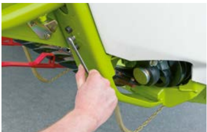
You can easily adjust the crop divider for height with the panel key.
