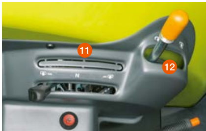
The PTO is engaged with hydraulic support as standard. Electronic PTO engagement is available as an option in machines with REVERSHIFT.
