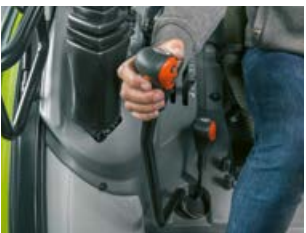
With REVERSHIFT: the electronic clutch is operated by pressing a button on the gear lever
