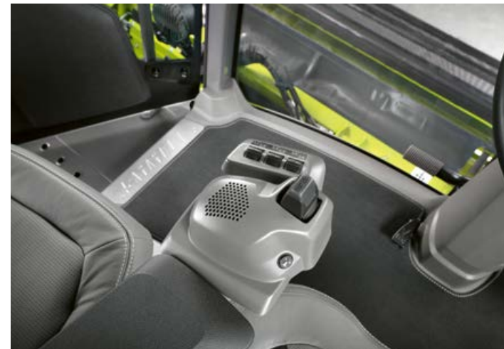
▲ Manoeuvring has never been more straightforward or effortless: the steering joystick and freely programmable function buttons are situated on the left-hand armrest. Page 40
