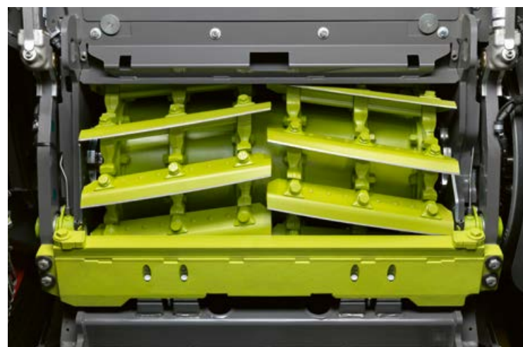
▲ The 910 mm wide V-FLEX chopping cylinder cuts cleanly and precisely. Flexible configuration options allow the cylinder to meet extremely varied requirements. Page 22
