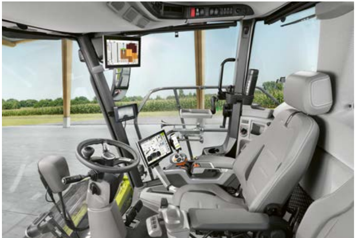
▲ High comfort, low noise level, excellent all-round visibility: the spacious cab mounted on silent blocks provides a pleasantly stress-free working environment, even during long days in the field. Page 38
