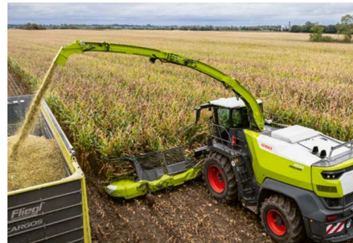
▲ The wider front attachments, such as the 14-row ORBIS 10500, maximise conversion of the engine output into throughput. Page 14
