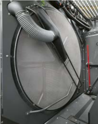
▼ The extractor fan operates continuously during field work and road travel.
