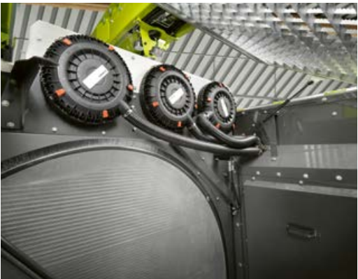
▲ The three air filters which ensure a reliable supply of air to the powerful engine can be accessed without tools for fast maintenance.
