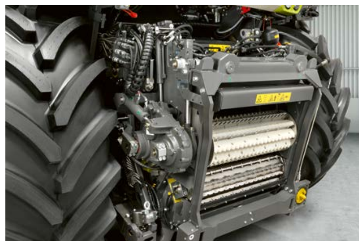
▲ The fully hydraulic pre-compression enables high throughput in all crops and lengths of cut while maintaining uniform chop quality. Page 20
