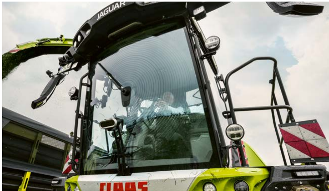
▲ The premium windscreen wiper with integrated screenwash spray provides perfect visibility, even in very difficult harvesting conditions.
