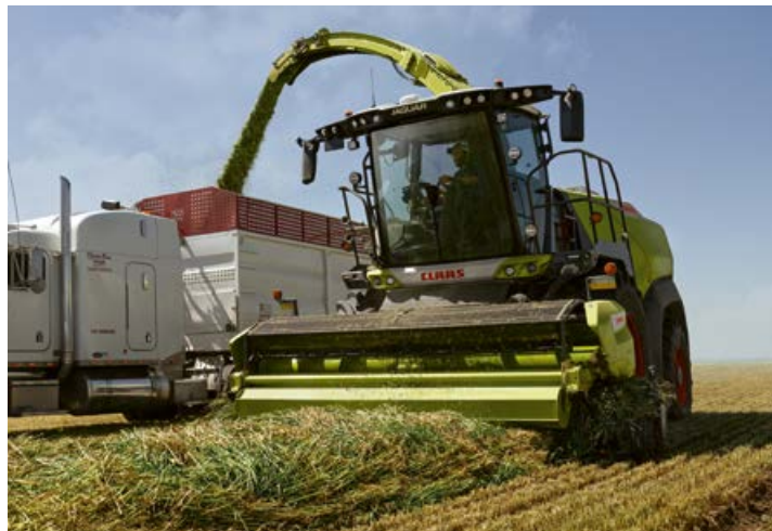
▲ High-performance front attachments like the new PICK UP, which provides an unrestricted feed with no overload protection, increase your harvest performance significantly. Page 16
