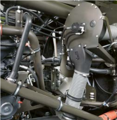
▼ The extractor fan operates continuously during field work and road travel.
