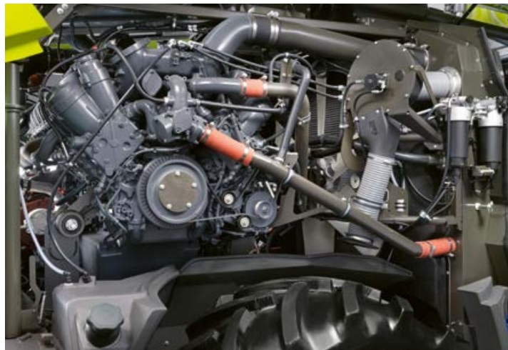
▲ The transverse engine transmits the huge output of up to 1,110 hp directly and efficiently. The output is ideally matched to the wide crop flow and the front attachments. Page 34
