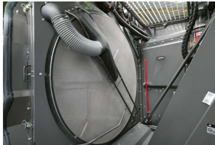
▲ Keeps cool up to 50°C. DYNAMIC COOLING applies only as much cooling as the JAGUAR needs at any time. An extractor system cleans the radiator screen continuously during field work and road travel. Page 35
