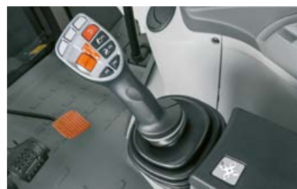
With the multifunction control lever, even FLEXPILOT spool valve operation is conveniently at your fingertips.
