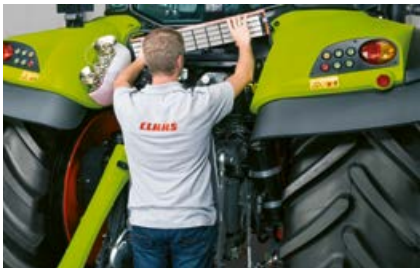
The cab air filter is behind the cab where it is easily accessible.
