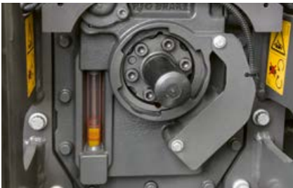
You can check the transmission and hydraulic oil level in a sight glass next to the PTO.
