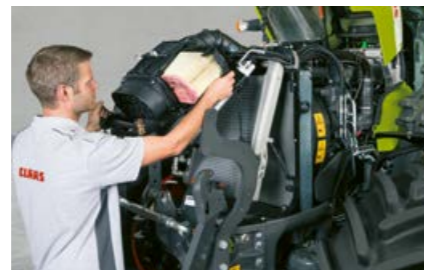
The engine air filter is located in front of the radiators and is easy to clean.
