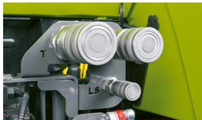
Power Beyond connections for the load-sensing circuit are provided at the rear for implements with their own control units. The implement then controls its own oil requirement, making permanent oil circulation unnecessary.
