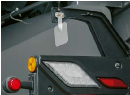
Sensor for automatic discharge direction adjustment
