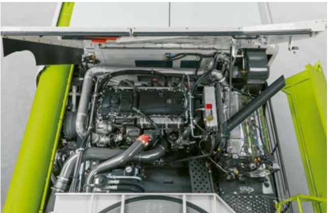
Mercedes-Benz OM 470 with 300 kW / 408 hp for LEXION 6700
