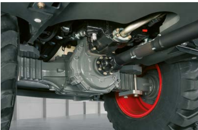
Hydrostatic transmission with self-locking braking action
