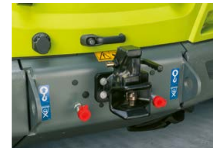
TORION 956 SINUS optionally with a pressure-free hydraulic return at the rear
