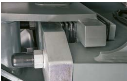
Rubber dampers in the articulated pendulum joint increase operator comfort
