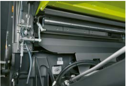
The large stone trap can be opened and emptied easily.
