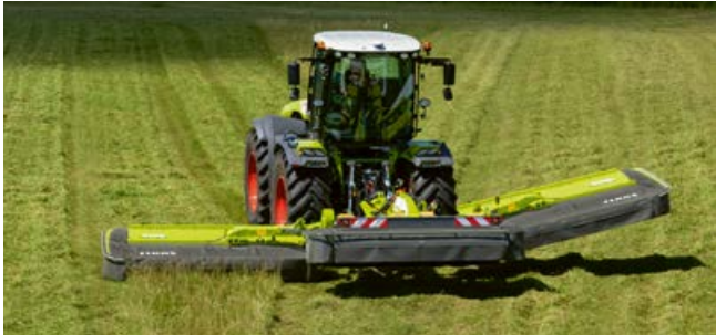
Individual mower unit lift at the headland
