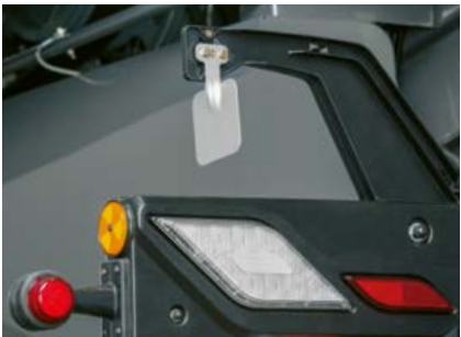
Sensor for automatic discharge direction adjustment
