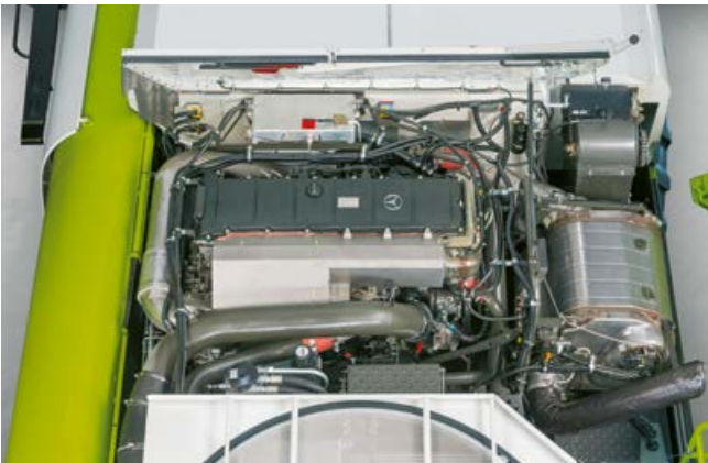
Mercedes Benz OM 473 with 460 kW / 626 hp for LEXION 8700
