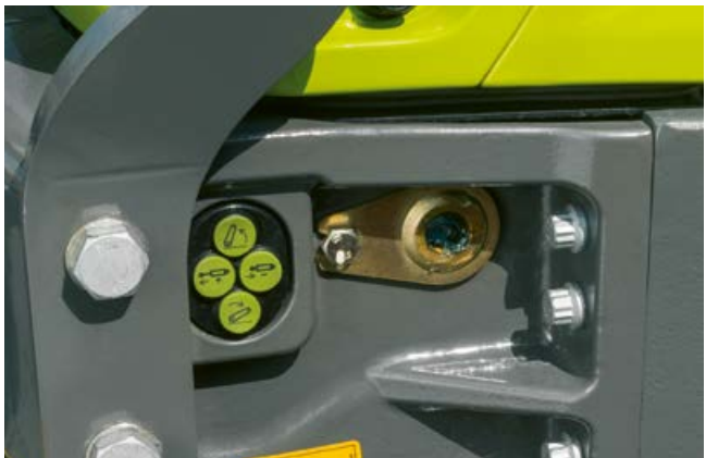
With electronic spool valves, the front linkage and additional spool valve can be controlled externally.
