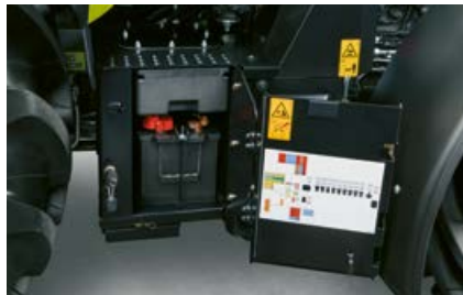
The battery, tool box and compressed air connection are located on the right side of the steps for easy access.
