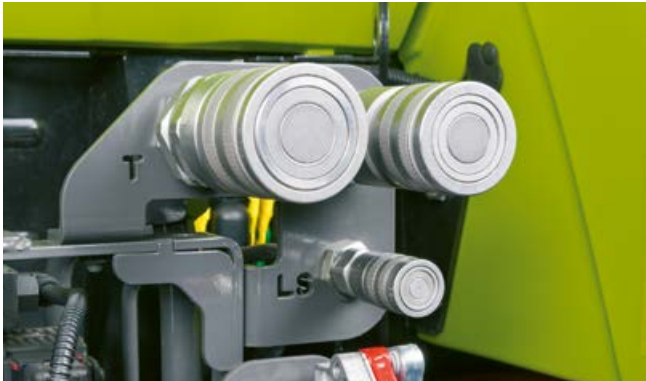
Power Beyond connections for the load-sensing circuit are provided at the rear for implements with their own control units. The implement then controls its own oil requirement, making permanent oil circulation unnecessary.
