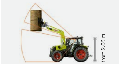
High-profile cab with transparent sunroof: minimum clearance height of 2.66 m.
